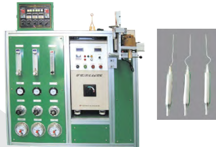
Thermo sensor tube brazing machine with inert atmosphere.
