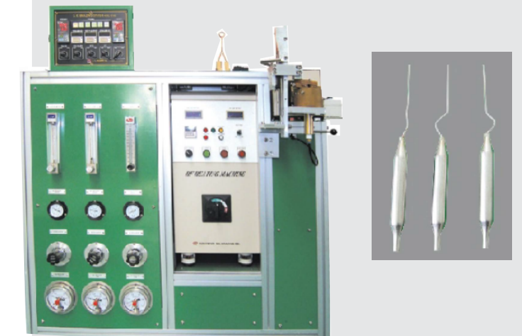
Thermo sensor tube brazing machine with inert atmosphere.
